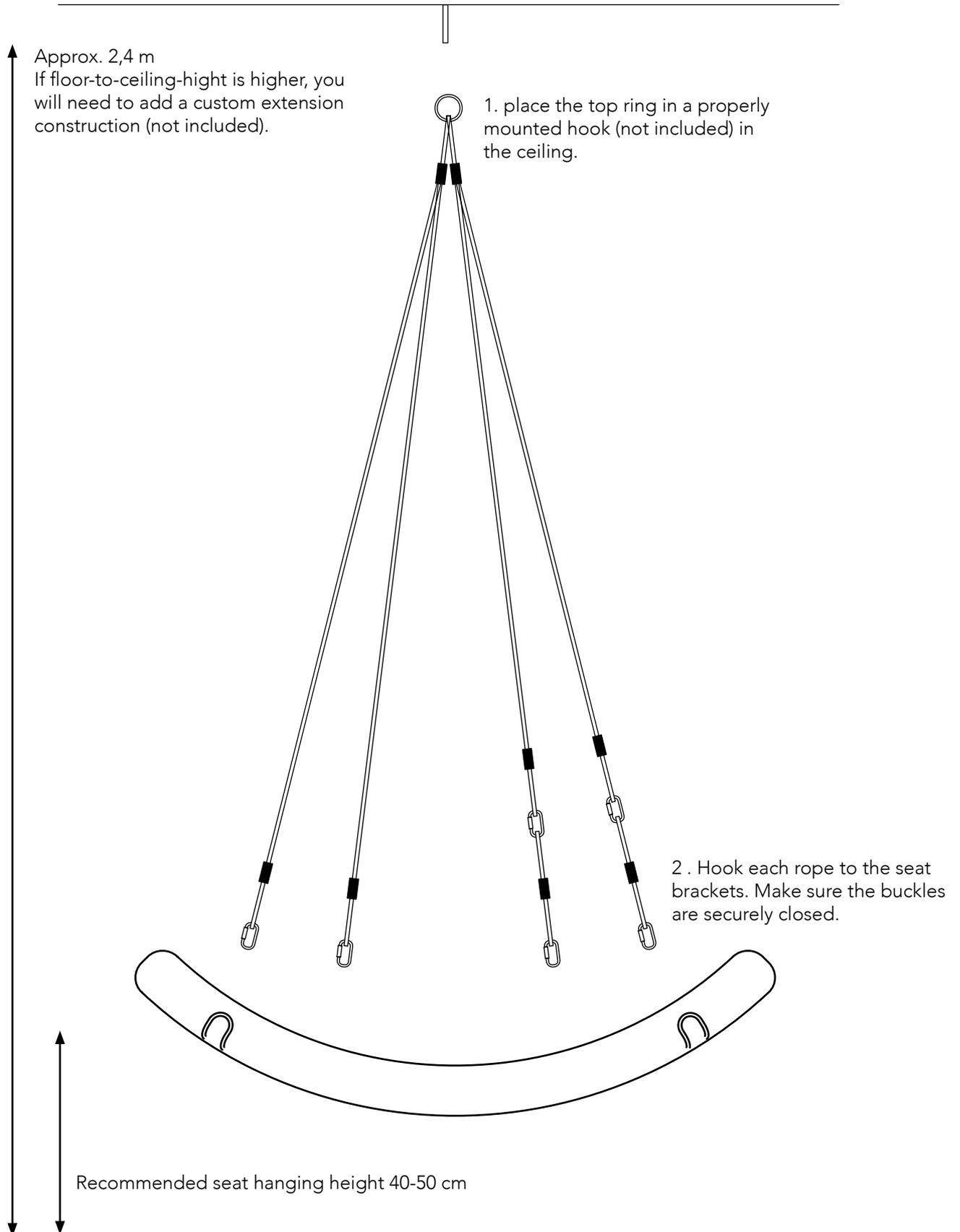
Make sure the buckles are securely closed with the nut. A wrench can be used to fully open and close the buckle.
